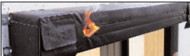
Fire-retardant foam isn't designed to keep a fire from starting.
