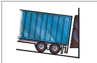
Tapered pads are best for sloped approaches.
